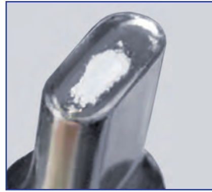
Granulate sticking to punch tip face
