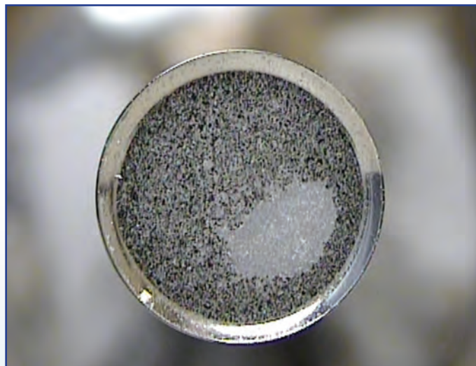
Granulate sticking to plain punch tip face.
